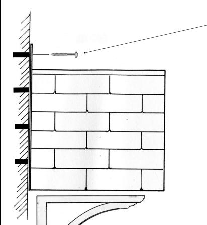
Apex canopies are normally fastened to the wall by fastening throu the GRP flange, using 65mm 10gauge (preferably stainless steel) screws at 300mm centres into suitable wall plugs and should then be finished with a lead flashing
