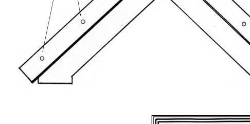
If required for either appearance or added support gallows brackets can be fitted to each side of the canopy. (For fastening of gallows brackets, see Gallows Bracket Fastening drawing)
